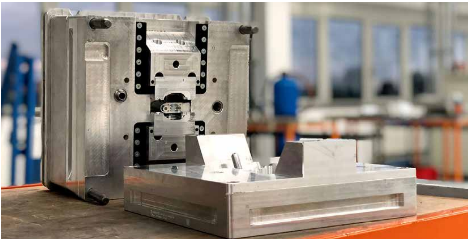
Aluminium mould in plastic injection moulding
